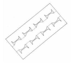
2 The documents in support of the priority claim described the design as a 'pasteboard tape with latching openings made from multi-ply cardboard, designed for holding together consumer packages, particularly bottles or cups into string sets of any length, which is spatially formed into a handling clamp and contains a cover separated by two folding lines from side walls where along both folding lines are cut-outs symmetrically disposed, each of which is provided with a latch wing, as
